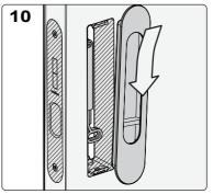
Insert the flush pull with the slide lock into cavity on the chosen side of the door. Push in and down so it grips onto the bottom bracket or edge.
