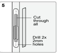
Mark the third rebate outline. Cut through into flush pull cavity.
