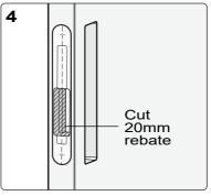
Place middle section of template into rebate and mark second rebate outline. Ensure it is the correct way up. Cut 20mm rebate
