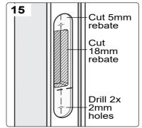
Place middle section of template into rebate and mark second rebate outline. Ensure it is the correct way up. Cut 18mm rebate
