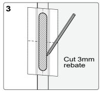
Remove middle section of lock template and mark rebate outline on end of door. Use midline as height reference. Cut 3mm rebate.
