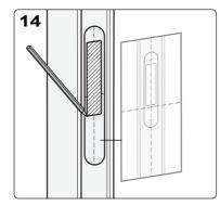
Remove middle section of striker plate template and mark outline for rebate. Use midline as height reference and ensure it lines up with the door. Cut a 5mm rebate.
