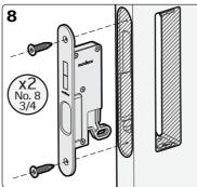
Insert the Privacy Lock assembly and secure with two No.8 3/4screws.
