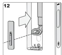
Insert emergency release onto the spindle.
