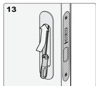
Insert second Flush Pull (Emergency release side) ensuring the Emergency release fits into the vertical slot on the back of the Flush pull .
