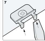
Fix bracket in centre of the cutout, ensuring that the tabs are hanging off the lip of the cutout. This ensures correct positioning.
