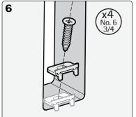
For wooden doors: install two woodfix brackets at top and bottom of cutout on both sides of the door.
