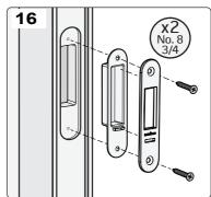
Insert striker plate assembly and secure with two No.8 \(^3\) screws.
